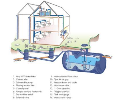
Figure 4.3-6 Example Rainwater Harvesting System in a Commercial Property
